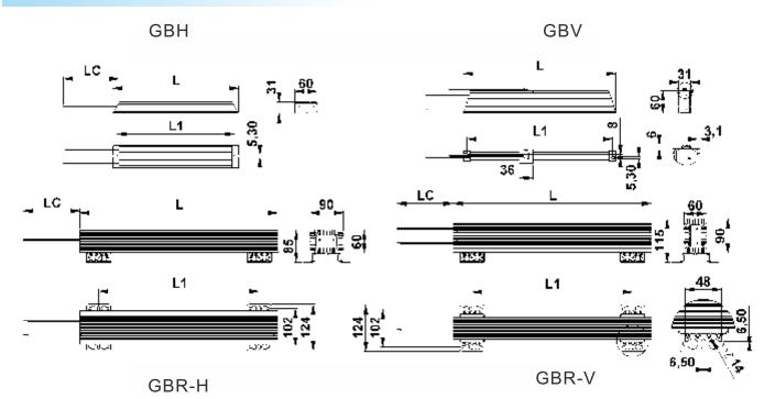
The external CLIP-ON thermo watch shown on GBV is also available for GBH. Internal thermo watch require 25 - 35 mm longer resistor profile, please require special data sheet.
