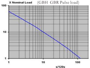
For further optimization offers KWX individual thermal electric circuit models for all types and ohm values. With these models can the temperature of the resistor wire and resistor surface be simulated during any pulse load conditions with a standard soft ware like Pspice. Alternatively offers KWX to make the thermal simulation for our customers
