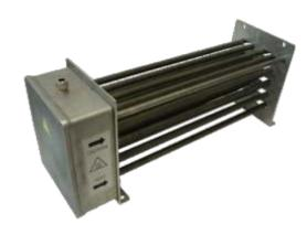
GRT style resistors are medium to high power resistors for con-stant load as in Filter applications and long braking cycles (example cranes). The GRT is constructed with Ø16mm tubular resistor elements, bended in U-shape and welded into two supports. On one side there is the electrical connection box in IP65 or higher.
