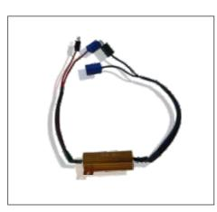
Aluminum Resistor is also called metal aluminum resistor, non-induction aluminum resistor, golden aluminum resistor, LED aluminum Resistor, etc.according to different applications and customs. Aluminum alloy shell with grooves on the surface for better dissipation. Owning small size, high power rating, resistance to high temperature and high over load, high precision, high stability, strong construction, favorable mechanical protection, easy nstallation, etc.
