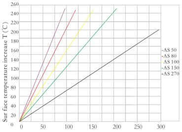
Fig: 3: Surface temperature increase vs. power for AS(2)
