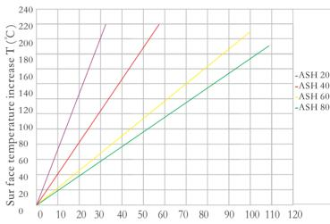
Fig:4:Surface temperature increase vs. power for ASH
