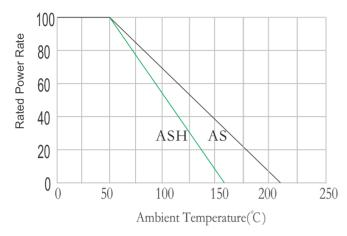
Fig:1:Derating Curves for AS and ASH
