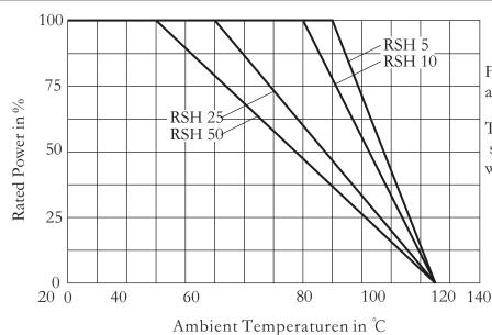
For resistors mounted onto heatsink and thermal resistance of 1 ° C/W.
